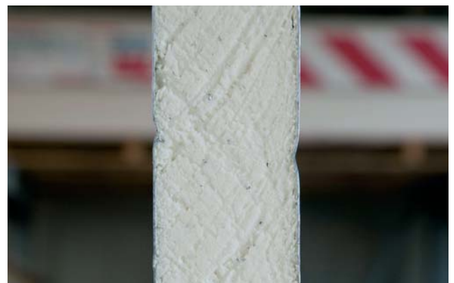
50 mm panels made of PU foam
