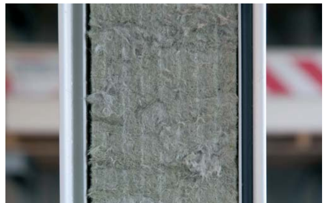
100 mm panels made of rockwool
