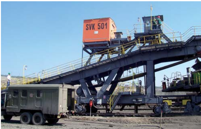
Container with transformer in open pit mining of brown coal
