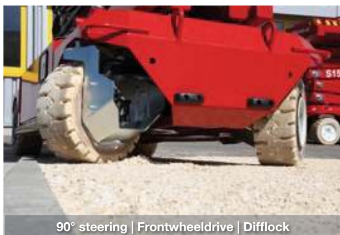
S171-12ES outdoor | 16KN vertical load
