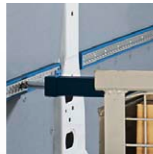
Lashing tracks on the loading room walls are ready to take cargo bars and secure the load with lashing straps
