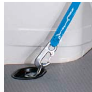
Thanks to the flush lashing points fitted countersunk in the Sobogrip floor, all standard lashing points provided by the manufacturer remain freely accessible
