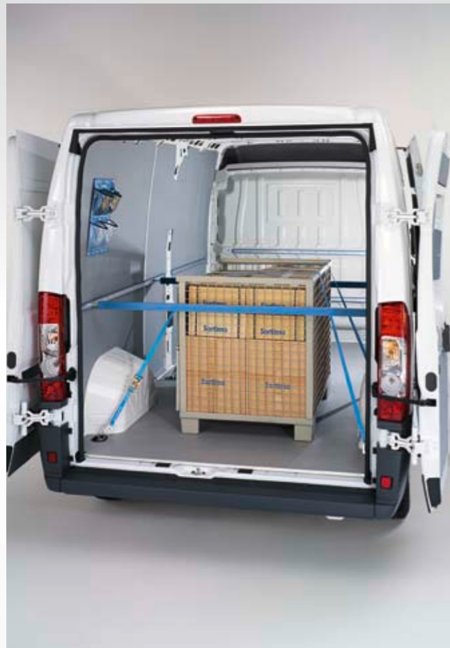
Lashing strap with ratchet to secure heavy cargo
