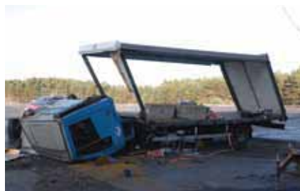
Terror Stopper 3 Bollard 273 x 10 V7500[N2]64-90-3.3-0.0
