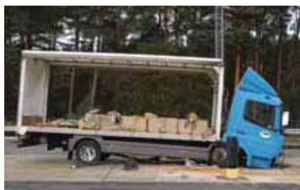
Terror Stopper 1 Bollard 219 x 10 V7500[N2]48-90-0.0-0.0
