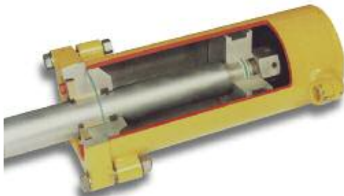
Coloured 'O' rings on a hydraulic cylinder.
