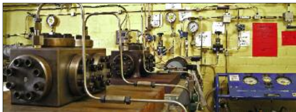
James Walker's eight-flange explosive decompression test rigs.
