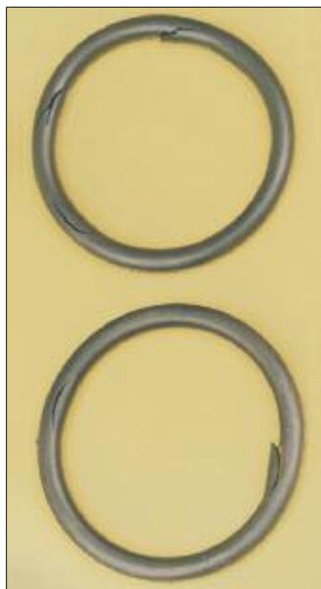
'O' rings after explosive decompression.
