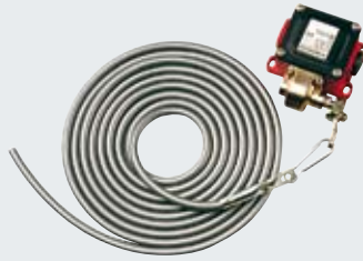
Pull switch with plastic pull cord Horizontal or vertical fitting possible, die-cast aluminium housing IP 65, cord length 4 m.
