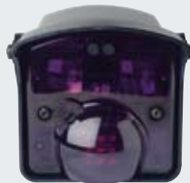
Comfort radar/presence detector Radar movement and presence detection with infrared detection. Quick and targeted automatic door opening. Reliable protection of the area in front of the door. Up to max. 6 m height. In areas with high levels of humidity and in outside areas, only the radar function is available. Housing: protection category IP 65
