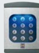
Radio code switch FCT 10b Using a radio code switch FCT 10b, you are able to transmit up to 10 radio codes (868.3 MHz). No laying of cables required. The keypad illuminates when initially pressed.
