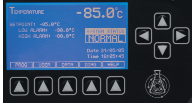
Large character display provides immediate review of important parameters "at a glance" from a distance. Intuitive menu system and directional arrows provide simple access and control of all parameters.
