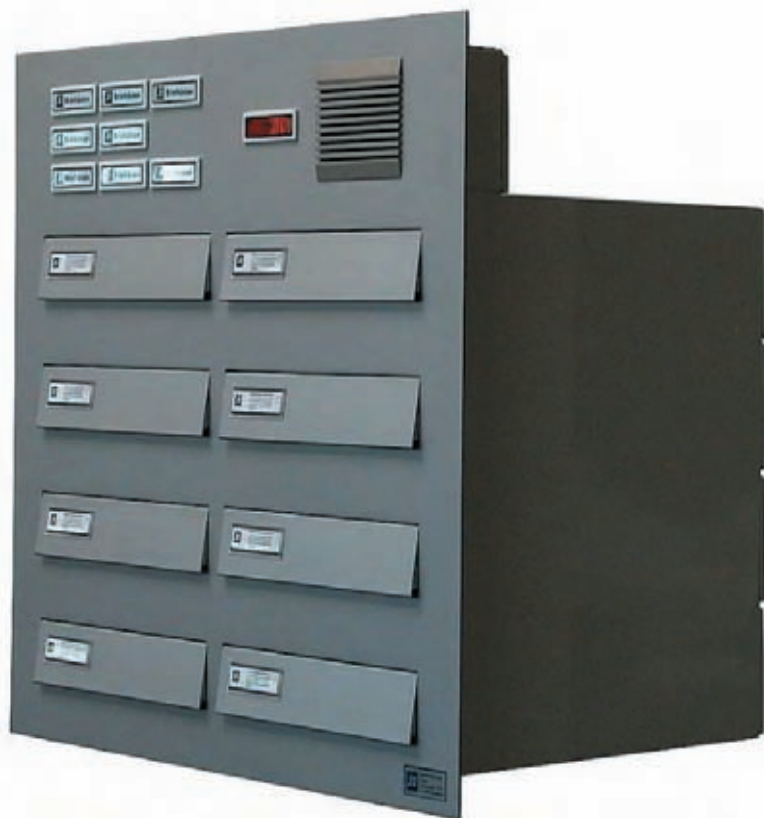
Bank with straight boxes and installation box for entrance panels. Frontplate and flaps made of aluminium. Powder coated in RAL 9007 grey aluminium.
