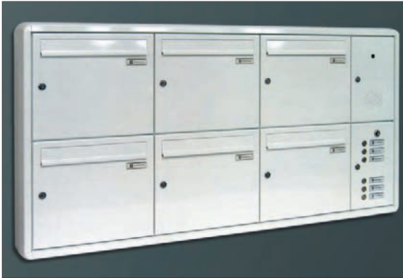
Bank for wall mounting 04-600 series with aluminium round profile section 20-243N. With installation box and accessories bellpush 21-117, name plate 21-255, illumination button 21-118 and punched speechgrille 21-165.
