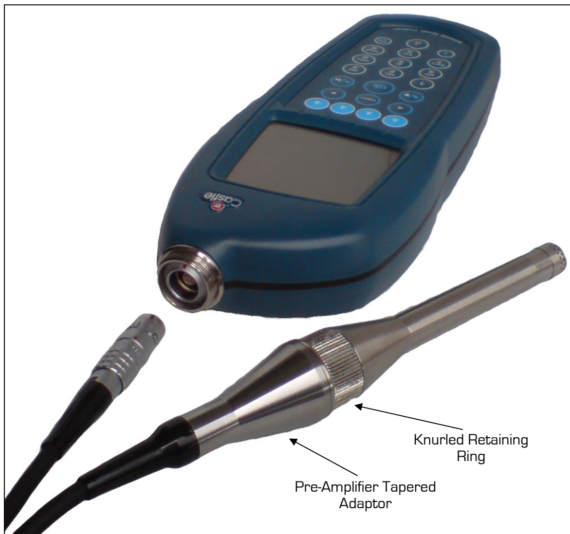
Figure 2 - Attaching and Removing the Microphone Extension Cable
