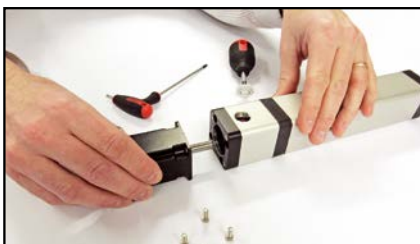
Insert motor shaft into coupling
