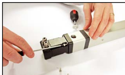
Tighten motor mounting screws
