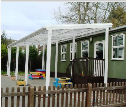
Freestanding Meridian Canopies positioned adjacent to the schools, where the buildings do not have either sufficient height or structure to support a standard lean-to Meridian.
