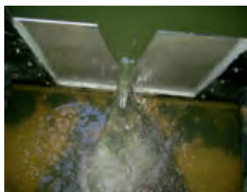
V-Weir The weirs are calculated by us. Various shapes possible.
