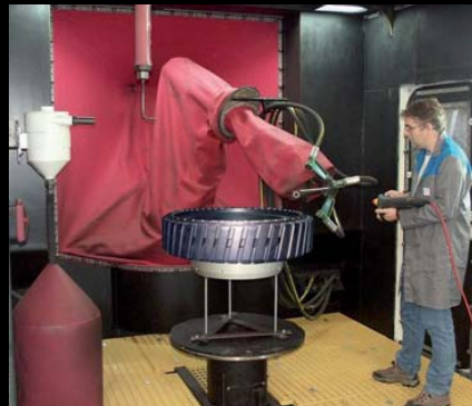
Inside view of the MPR 1800 shot peening cabinet
