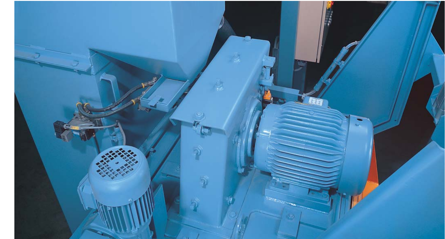
Directly driven blast wheel
