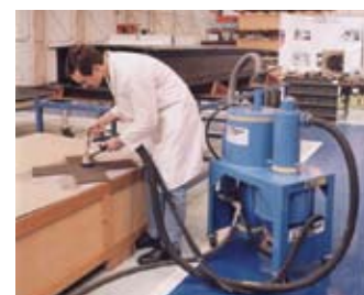
Preparation for bonding on composite materials
