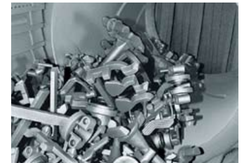
Parts in the outlet barrel after cleaning
