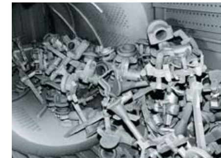
Uncleaned castings in the inlet barrel
