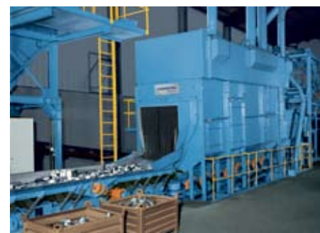
The DT 14 throughfeed blast cleaning machine for economical, low-pollution, non-hazardous operation
