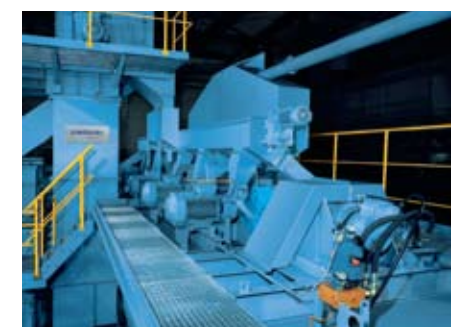
Cabin top of a DT 14-1050 equipped with 10 blast wheels
