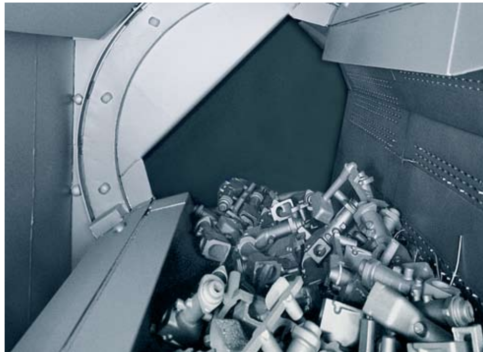
Castings within the blasting zone of the machine
