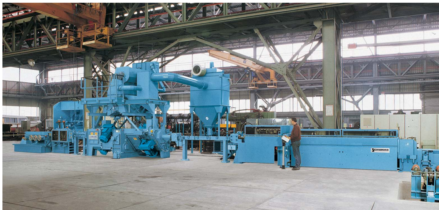
Shot blast machine with dust collector
