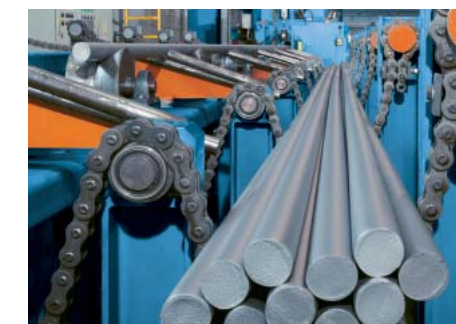
Blast cleaning machine for longitudinal wire descaling
