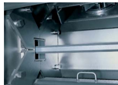
Shot blast chamber
