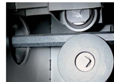
Pressure-rollers guide the workpiece
