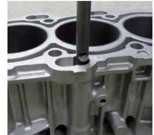
Inside blasting of crankcases
