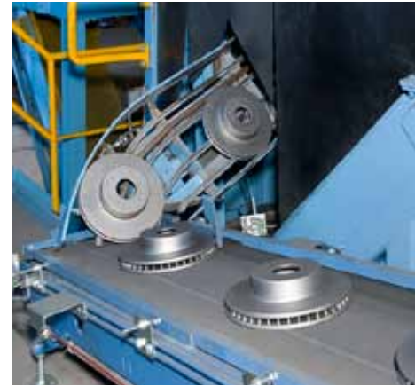
Process-safe blasting of single parts
