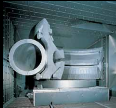
Blast cleaning (sand removal) of compressor housing
