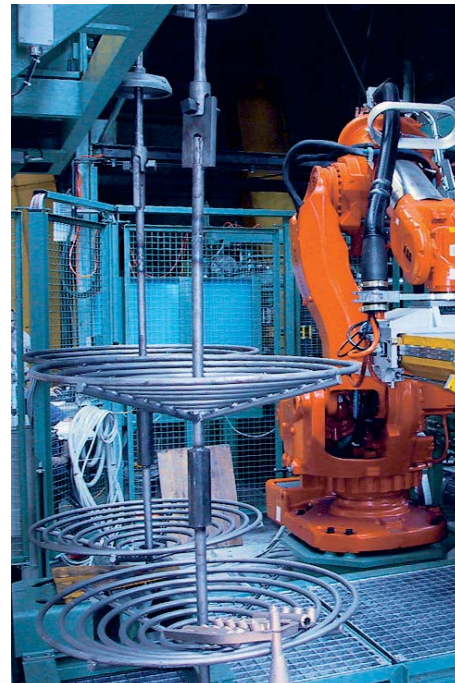
Robotic loading of hangers
