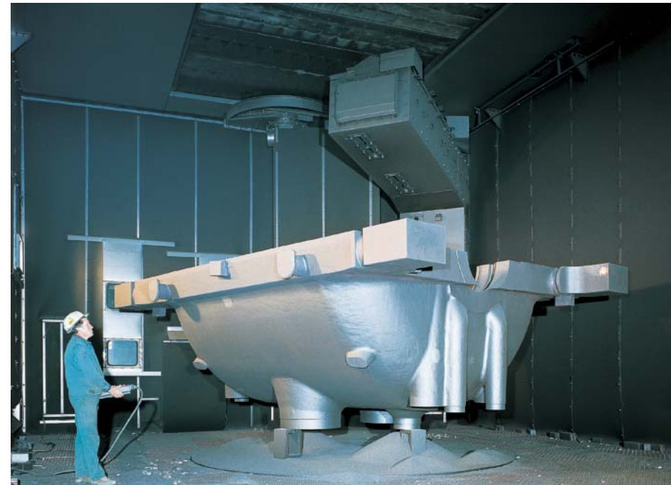
Blastroom with wheels on a tower
