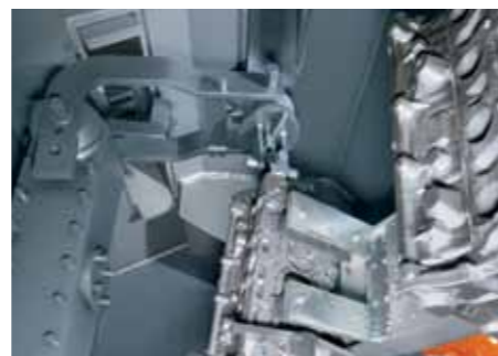
The double manipulator assembly permits loading and unloading within seconds
