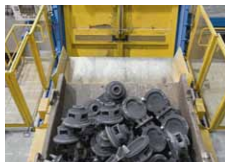
Loading /unloading of heavy parts in a foundry
