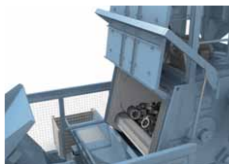
Hydraulic loading, discharge via vibratory conveyor
