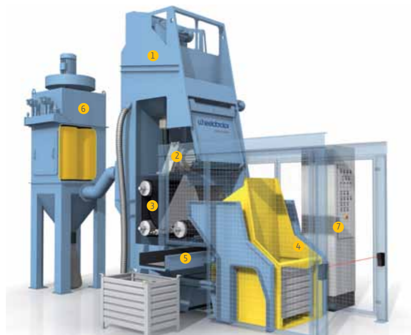
MB Tumbblast machine with hydraulic loader and dust removal system
