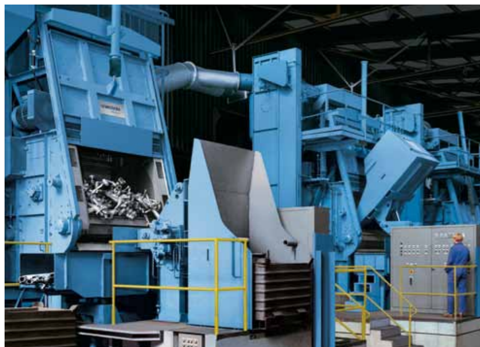
Shot blast machines in a foundry
