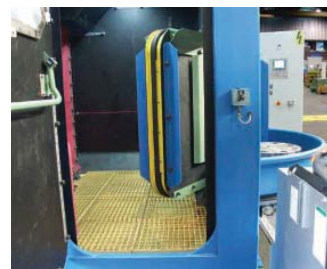
Revolving door with inflatable seal
