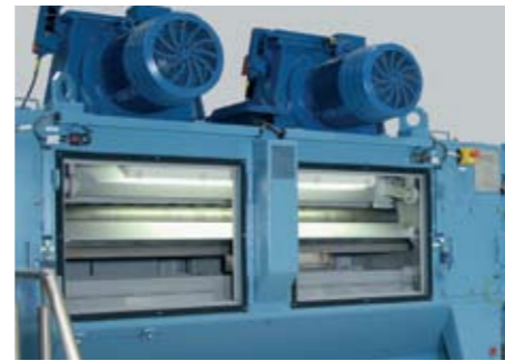
Blast room, transport rollers
