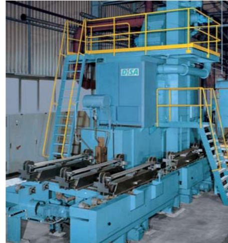
Leaf spring stress peening system.
