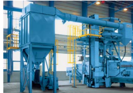
Shot peening and exhaust system at manufacturer's works
