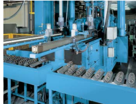
Unloading side of the shot peening system.
