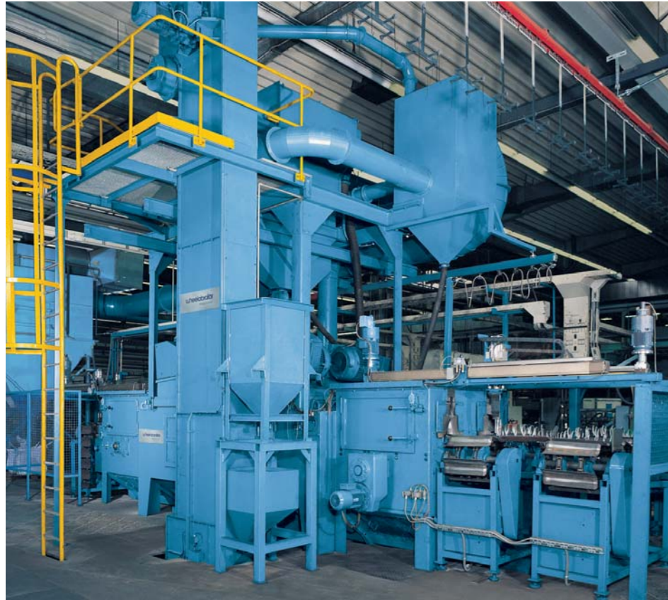
Coil springs shot peening system with 4 blast wheels.
