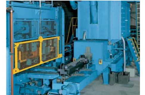
System for stress peening leaf springs
