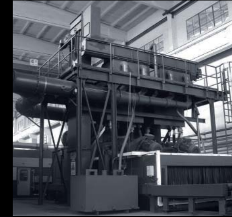
Roller conveyor shot blast machine
