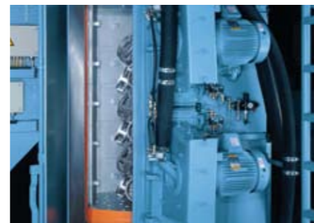
SPH 2-5,5/12, rear of machine with blast wheels, maintenance access door open
