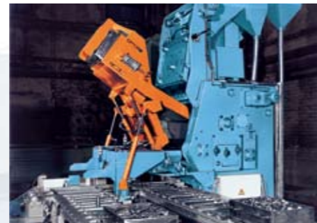
Shot blast machine with automatic loading and unloading system
