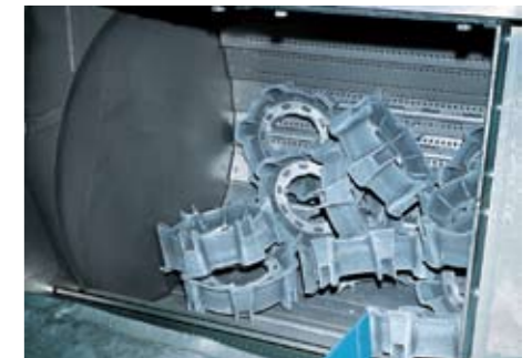
Even large parts can be perfectly shotblasted
