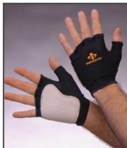
502-10 Fingerless style for all purpose with hand or electric tools. Suede leather and VEP padding in the palm. Sold left, right or pair.
