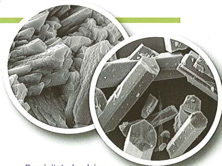
Precipitated calcium - Untreated (left) and treated (right)
