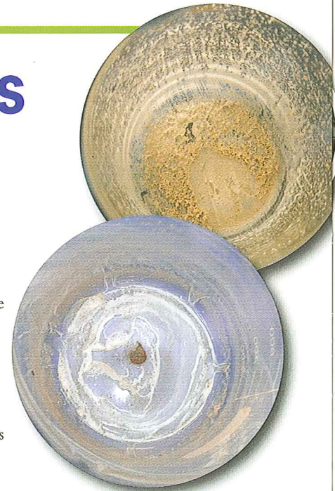
Minerals in steam carry over before (top)... and after (above) treatment
