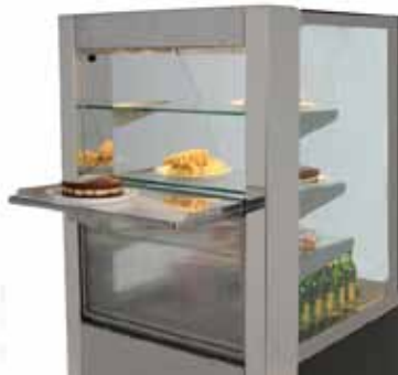
Drop-down top doors form load bearing shelf and direct cold air under the mid shelf preventing it from escaping when the doors are open.
