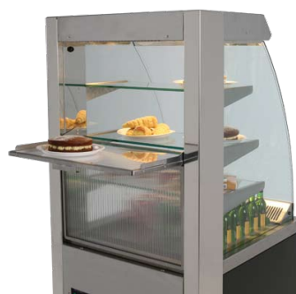
Drop-down top doors form load bearing shelf and direct cold air under the mid shelf preventing it from escaping when the doors are open.
