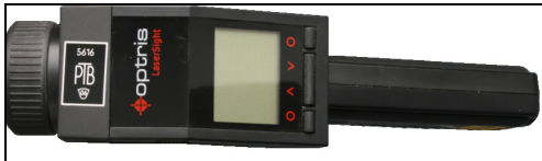
Transfer standard IR thermometer LS-PTB
