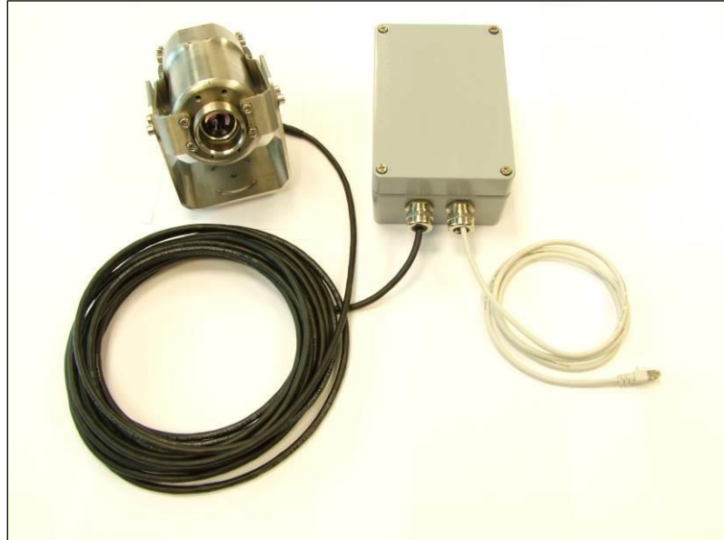
IR camera inside CoolingJacket, connected to a NetBox via high temperature USB cable
