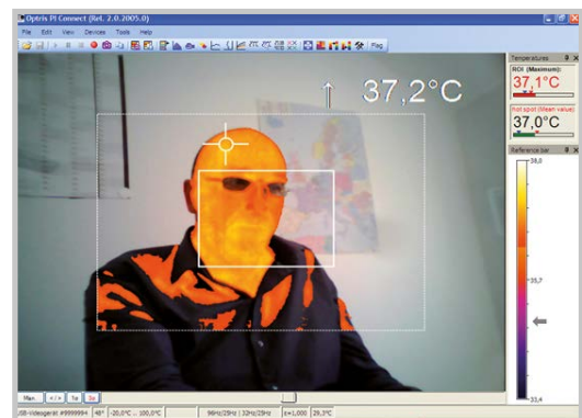
Cross-fading of VIS image above temperatures of 35 °C
