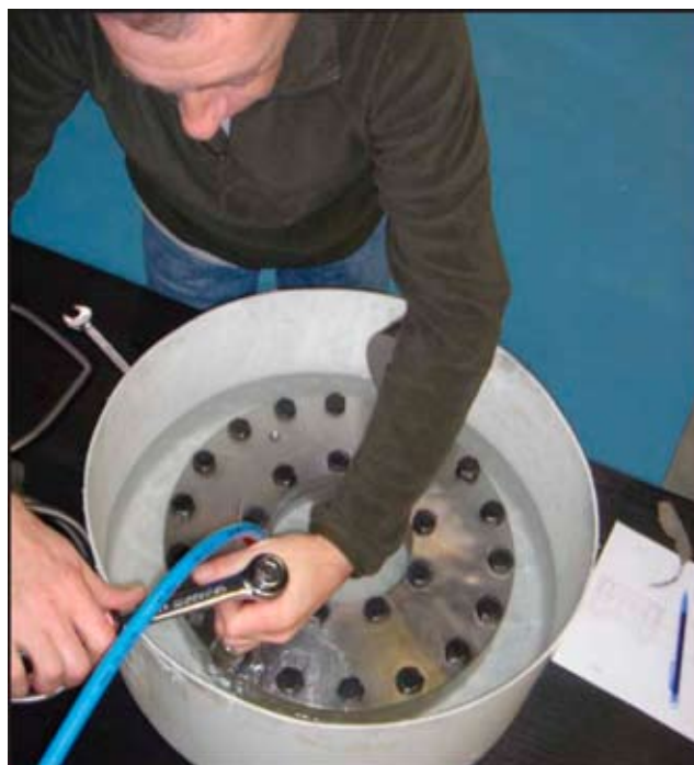
Custom built leak test
