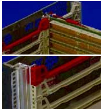
2 slots per U for CPCI/VME boards at the front and rear.
