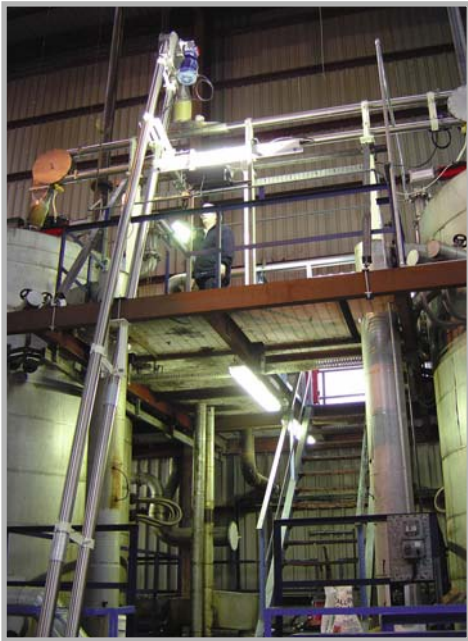
Aero mechanical conveyors are ideal for difficult products such as titanium oxide and other products which have tendency to smear or are cohesive.
