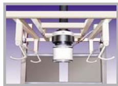
Optional automatic bag loop release.
