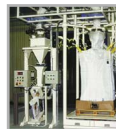
Using the same basic filling platform, special adaptors can be supplied to fill product in to other types of containers such as rigid IBCs, drums and tubs.
