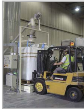
Optional automatic bag loop release.
