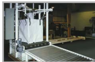
Using the same basic filling platform, special adaptors can be supplied to fill product in to other types of containers such as rigid IBCs, drums and tubs.
