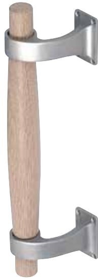
ATSSHA86-304 Stainless steel & oak offset handle Height 400 Backplates 69 x 40 Projection 93 Ø44
