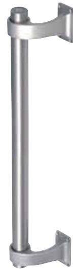
ATSSHA84-304 Stainless steel offset handle Height 400 Backplates 69 x 40 Projection 93 Ø32
