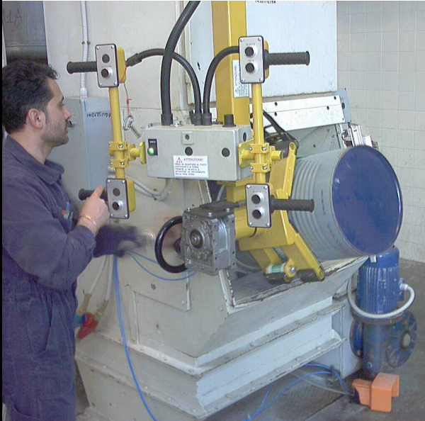
Industrial manipulator INDEVA for lifting and tilting drums.
