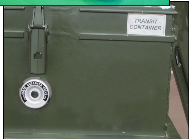
Pressure Relief Valve mounted to a transit container
