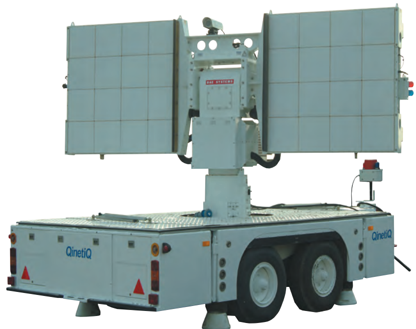
Panel antennas for CW Doppler Radar System, as front cover
