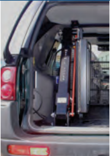
LoadLift specially developed to fit inside a Land Rover Freelander.
