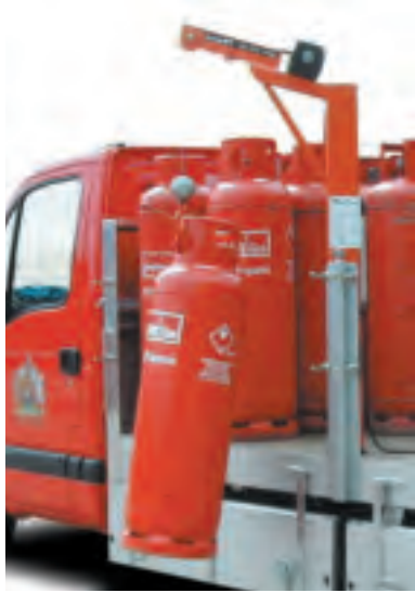
Gas bottle crane originally supplied to Calor Gas to increase safety and efficiency of small drop deliveries.
