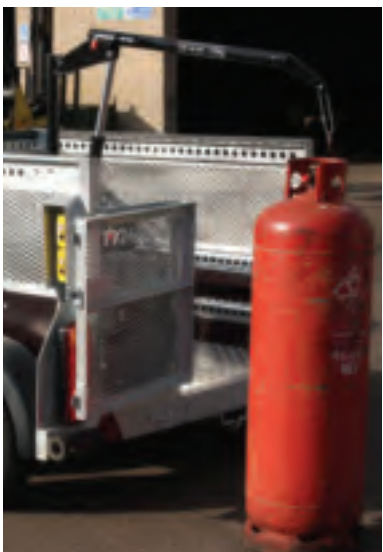
Gas bottle recovery trailer used by BOC as a fast response trailer to deal with spills, hazards and discarded gas cylinders throughout the UK.
