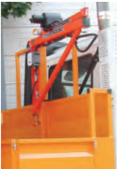
SwingLift two metre knuckle joint crane fitted to a "hot box" vehicle used for lifting and lowering heavy propane cylinders.
