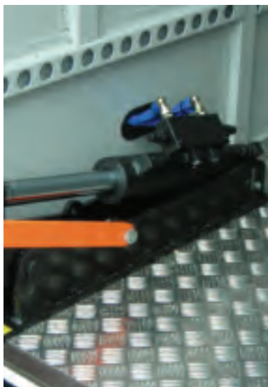
LoadLift (side door application) showing how the power pack can be remotely mounted under the passenger seat creating a spark-free environment and even greater load space.
