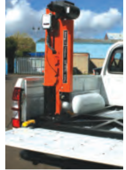
4x4 pickup complete with SwingLift F500 crane and SLF7 floor frame.
