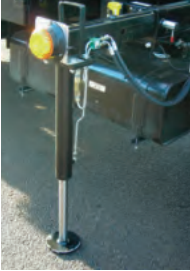
Hydraulic support leg with optional interlocks and warning lamps.
