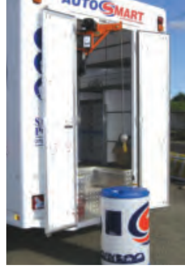
Corner crane, ideal for loading plant or chemical drums where space is at a premium.
