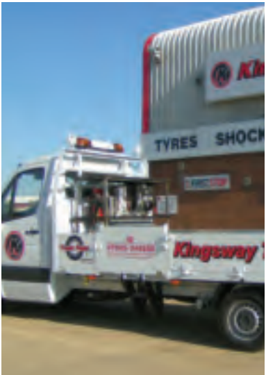
SideLift fitted to Kingsway Tyres VW Crafter - ideally suited to loading tyres away from the risks associated with working at the rear of the vehicle on busy roads.
