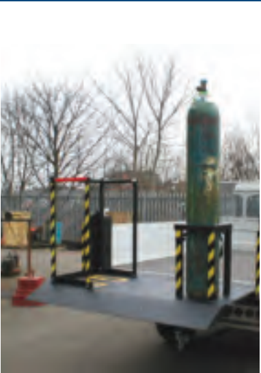
Easyloader TailLift and folding guard frames developed for Severn Trent Water.
