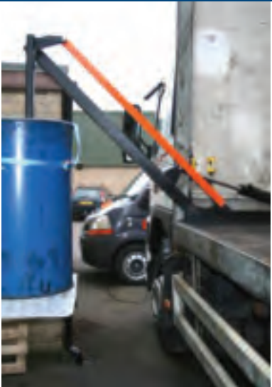
LoadLift fitted to 7.5t rigid for handling waste oil barrels.
