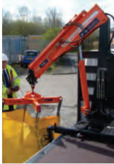
FV1200 showing how ideally suited this strong yet compact crane is for loading heavy items onto a 3.5t vehicle. With a 1.2 tonne capacity it will easily load and unload 1 tonne bags of sand.
