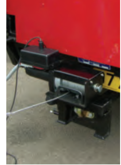
Penny Hydraulics WinchPack complete with remote control, integral solenoids and free spool.
