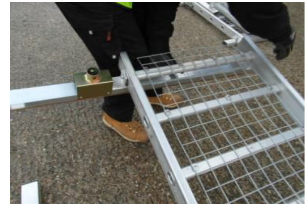
B. Attach the first support batten to the underside of the Board-Walk section using the captivated pins in the holes in the stiles (mesh side is the top)
