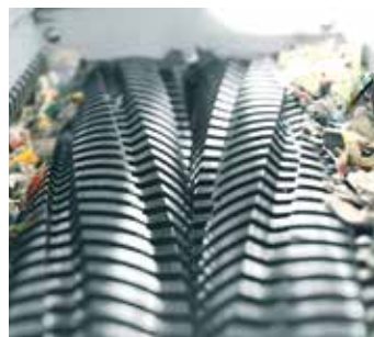
Cutting unit stage 2: downstream shredder
