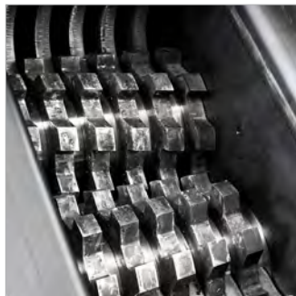
Specially hardened solid-steel cutting units manufactured from a single piece – robust, reliable and durable.
