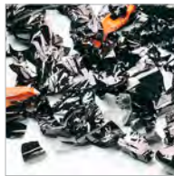
Particles of shredded magnetic tapes, credit cards and customer cards. Cutting size: 20 x 40-50 (<1000 m 2 ).
