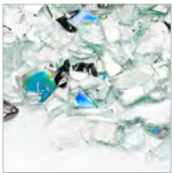
Particles of shredded CDs, DVDs, Blu-ray discs. Cutting size 20 x 40-50 (<1000 m 2 ).
