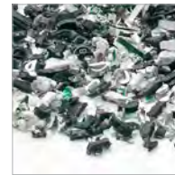
Particles of shredded USB sticks. Cutting size 20 x 40-50 (<1000 m 2 ).
