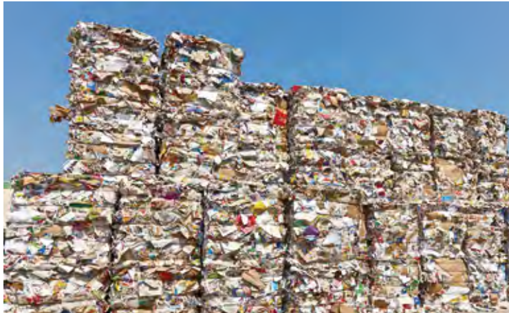
HSM presses can create bales of recyclable material weighing up to 1,100 kg
