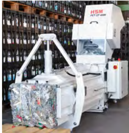
Crushing and pressing of PET bottles in a single work cycle
