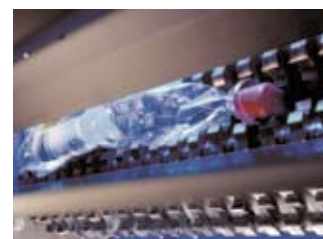
Dosing shaft for reliable feeding
