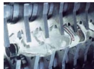
The special shape of the rollers - with large and small grippers - ensures reliable feeding of varying bottle sizes.
