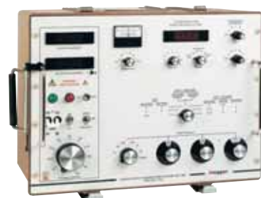
670000 comes complete with interference suppression circuits for testing in high-voltage switchyards, automatic balancing of dissipation factor, and direct readout of capacitance, dissipation factor and watts dissipated
