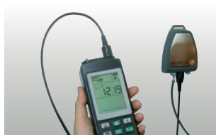
Inspection of transmitters with 4 to 20 mA interface
